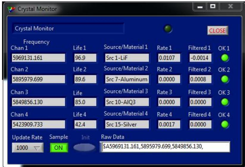
All 4 channels are sampled simultaneously. If the Raw Data is not updating on a regular basis pressing the green ON next to the Sample Update selector will interrupt the sampling and enable the Init button. Pressing the Init button will initialize the communication channel to re-establish communications with the crystal monitor.
