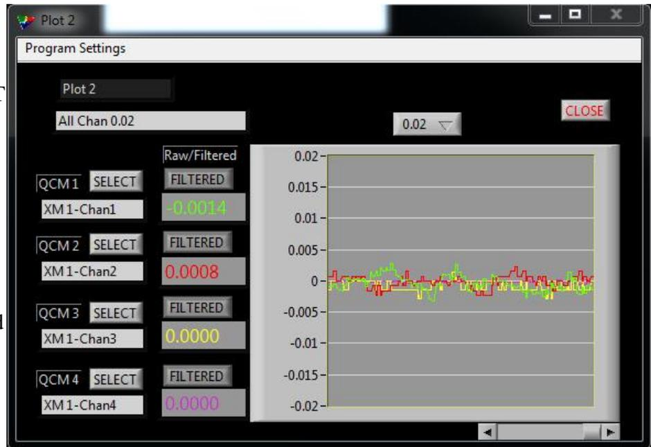
want to view one channel you can create a named setting with only that channel visible. The Program Settings selections include: Load, Save, Save As, Delete, and Rename. Load will read in the parameters that were saved previously. Save will save the new values to the current setting name. Save As will create a new setting with the name selected by the user. Delete will delete the settings from the list. Rename allows the user to change the name of a saved setting. NOTE: This dialog should be
